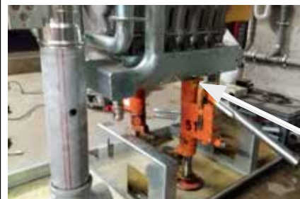
Male lifting piece on the return pipe
