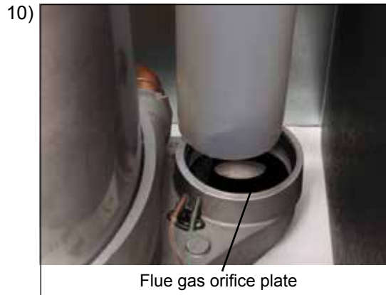
10) Place the Ø 53 mm flue gas orifice plate into the condensate pan and reinsert the flue pipe.
