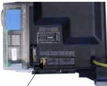
Break out the cover of slot no. 20 with a screwdriver or universal pliers
